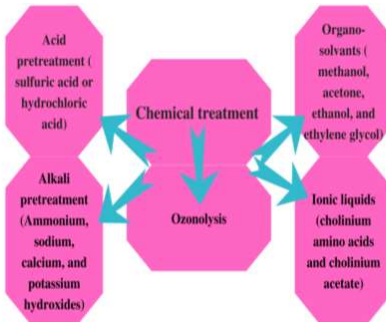
Figure 4. Different chemical pre-treatments of crop residues in order to improve cellulose availability and separation from the wastes through delignification process.
